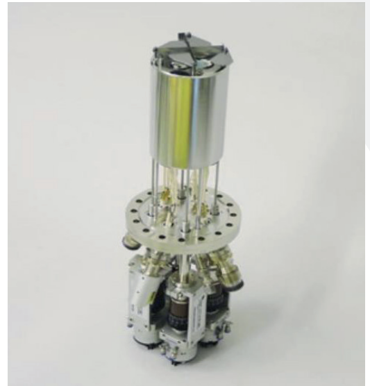
Quad cell OEZ 100-4x10-22-KS: Four 10 cm 3 crucibles on a single DN100CF (O.D. 6") flange, with integrated water cooling and rotary shutter
