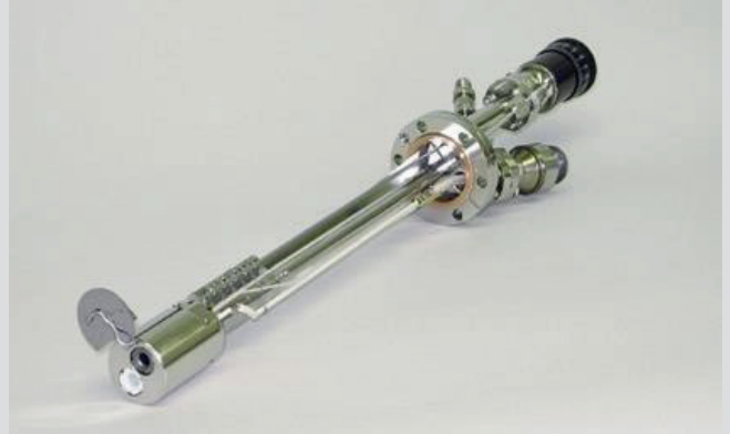
Dual cell OEZ 40-2x1-14-S: Two 0.6 cm 3 crucibles on a single DN40CF (O.D. 2.75") flange, with integrated water cooling and rotary shutter
