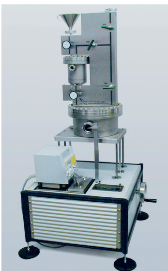
HGSU Control Unit for use with HGS source: electronic rack and table with liquid bath temperature controller and external reservoirs
